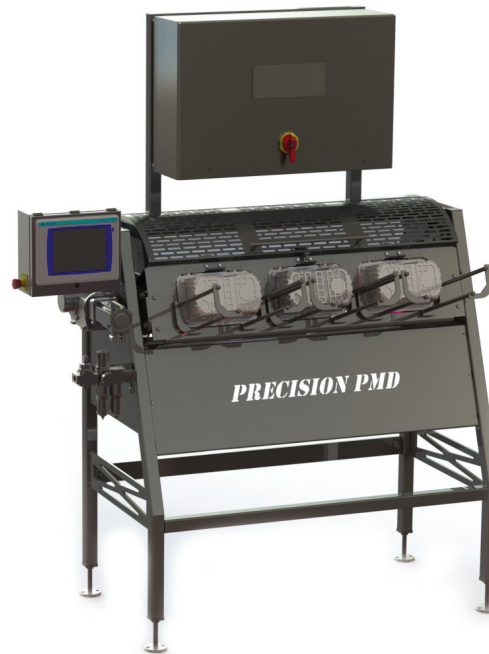
The new servo-driven Precision PMD vacuum denester boosts repeatability and speed.
