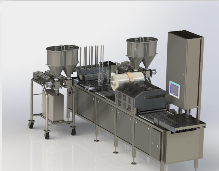
HEALTH FOOD PUDDING CUP Qty 2 - Two Head Piston Fillers Shown over a Precision PMD Four Lane Cup Packaging System including: Four Lane DNester, Membrane Sealer, Die Cutter. System speed is 180 cups per minute (3.5 oz fill).
