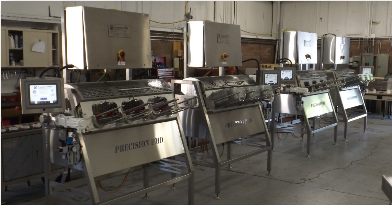
Shown Are Four (4) Precision PMD PNP Container Placement Systems All shown place three tubs per cycle, two run large tubs, two run small tubs. All tooling is interchangeable. Each system operates at 100CPM. (depending on configuration)
